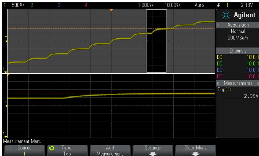
Figure 45 Isolating area for Top measurement
